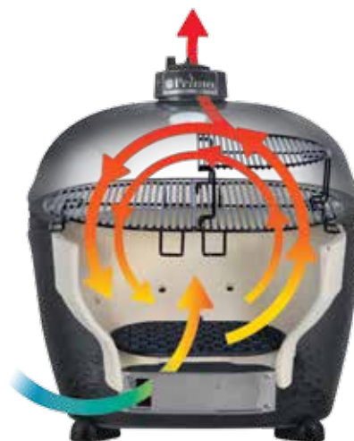
Cool air is drawn into the bottom vent, heated by the charcoal and convects around the food before exiting the top vent. The ceramic shell helps food retain its moisture.
