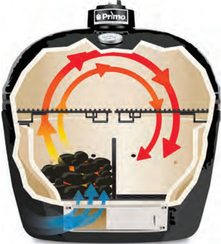
Cool air is drawn into the bottom vent, then heated by the charcoal. The heated air convects around the food before exiting the top vent. The ceramic shell retains more heat than metal grills, and helps food retain more of its moisture than conventional grills.
